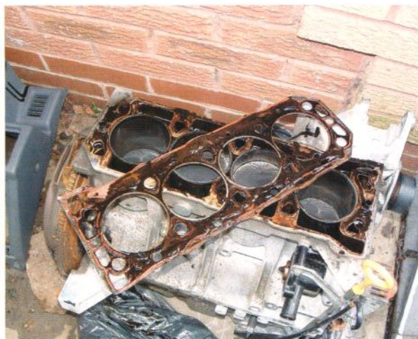
Fig. 4.32 The head gasket becomes a gooey mess.
