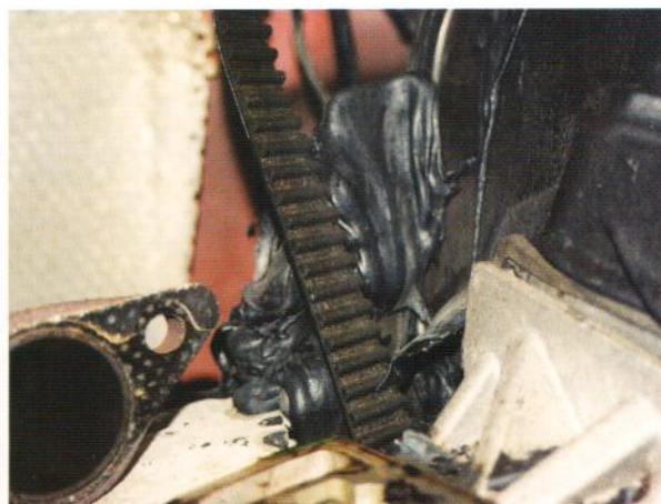
Fig. 4.34 This engine was run until it just stopped and all the plastics started to melt, with the cam cover reduced to a blob.
