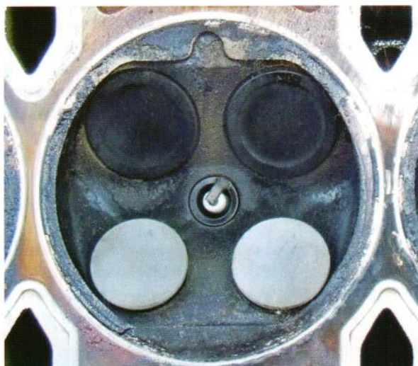
Fig. 4.75 Valves are close to the head face that restricts the maximum skim limit and on this MPI head with small valves there is more scope for skimming.
