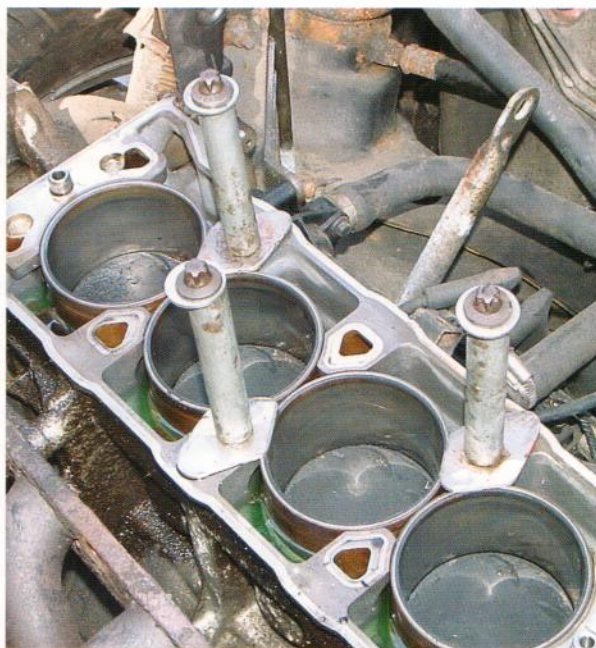
TOP LEFT: Fig. 4.71 Once the through bolts have been removed you must never turn a K series engine over unless you have fitted liner clamps to stop the pistons lifting the liners of their seats in the block and breaking the seals. (Austin Garages)
