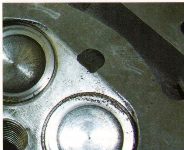
Fig. 4.78 A skimmed head looks like this. Some heads may even have seen the dimple completely skimmed away.
