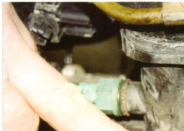
Fig. 4.37 Surprisingly, though, the plastic inlet manifold was just melting at the join onto the cylinder head.
