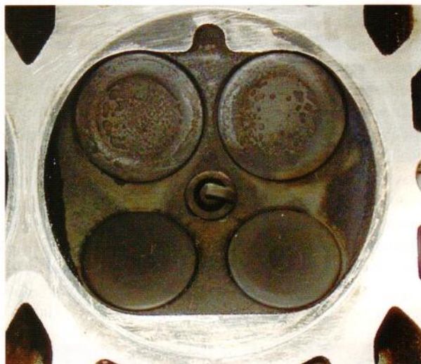
Fig. 4.76 On VVC heads, where the bigger valves are much closer to the head face, skimming is more of a problem.
