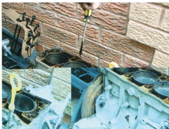
Fig. 4.31 When HGF is allowed to develop to the point where the engine stops, the coolant turns to a light tar.
